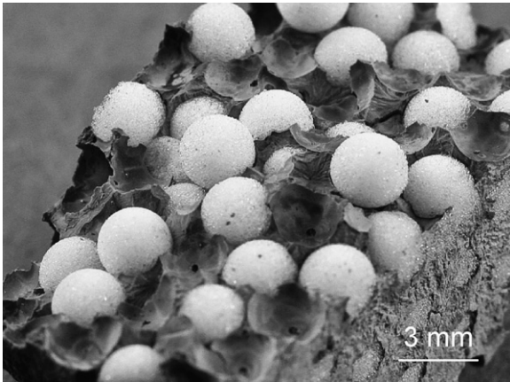
Fig. 9. Fracture facies of \text{CaCO}_3 scaffold filled with PMMA beads.
